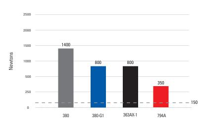
Test Method: ASTM D-5706, The test load is increased every 2 minutes until the specimens weld together, indicating lubricant failure.
