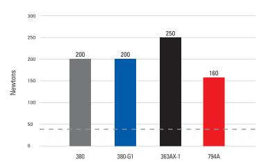
Test Method: ASTM D-2596, Measures the lowest applied load on Four-Ball Extreme Pressure (EP) at which the sliding metal surfaces seize and then load.
