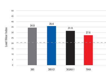
Test Method: ASTM D-2596, Creates an index of the ability for a lubricant to minimize wear at applied loads. It is based on a calculation of wear at non-seizure loads on the way to determining the weld point.
